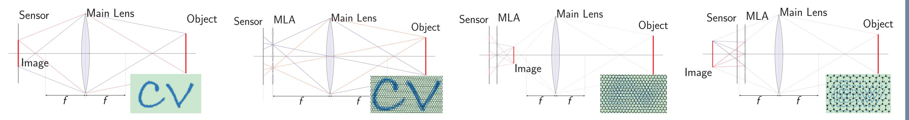
Figure 1: Comparison of optical design of a classic camera and plenoptic cameras. From *left* to *right*: classic camera, unfocused design (1.0), Keplerian design (2.0), and Galilean design (2.0).
